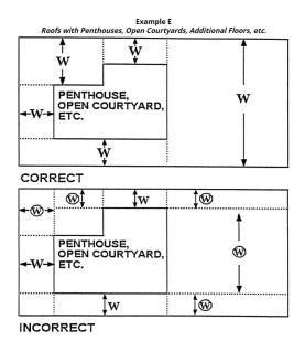
Such roofs are to be divided into subareas by using dividing lines of minimum length to minimize the size and number of the areas which are potentially less than or equal to fifty feet (15.25 m) in width in order to limit the size of roof areas where the safety monitoring system alone can be used. Dotted lines are used in the examples to show the location of dividing lines.
