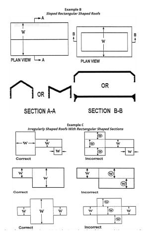
Such roofs are to be divided into subareas by using dividing lines of minimum length to minimize the size and number of the areas which are potentially less than or equal to fifty feet (15.25 m) in width, in order to limit the size of roof areas where the safety monitoring system alone can be used (WAC 296-880-40045(1)). Dotted lines are used in the examples to show the location of dividing lines.
